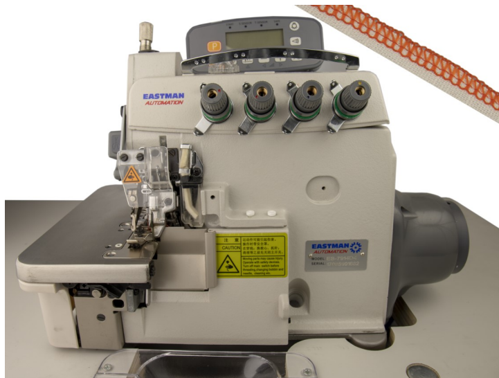
EA-7914D4 4 Thread Pneumatic Overlock Auto air suction & thread trimmer
